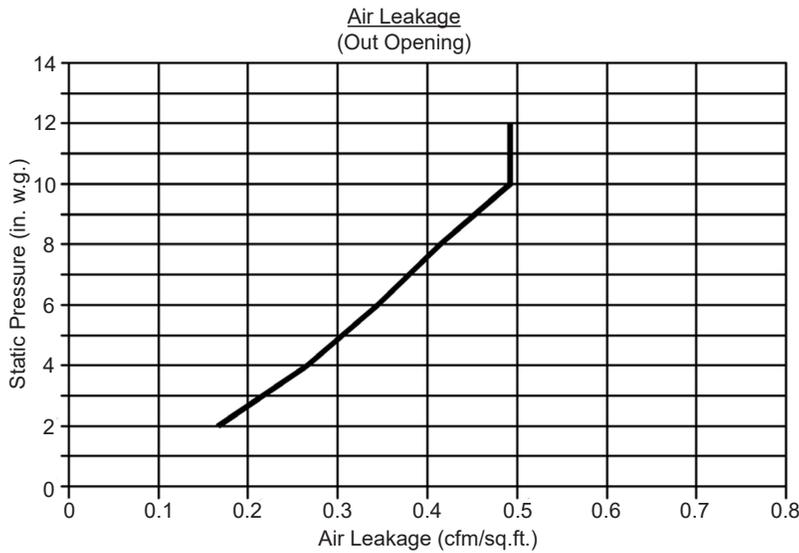
Air leakage chart is based upon independent air leakage tests conducted by Architectural Testing Laboratory. The out-opening model of a 26" x 60" AHF-T2 was tested. Tests were in accordance with ASTM E 283-91 "Determining the Rate of Air Leakage through Exterior Windows, Curtain Walls, and Door under Specified Pressure Differences Across the Specimen". Air Balance recommends using out of opening doors for draw through applications and in opening (IO) for blow through applications.
